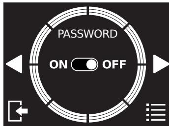
To set the password, it's necessary press **ON** and insert a 4-numbers code. After having pressed **CONFIRM**, you need to type it again and press **SAVE**.
