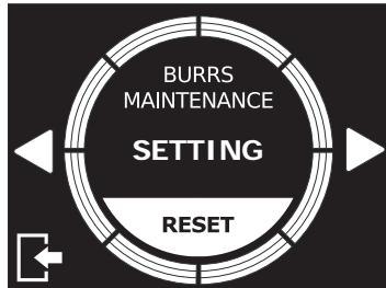
Pressing **SETTING**, you have access to the menu to enable/disable the burrs maintenance alert and you can set both the size and the type of the burrs.
