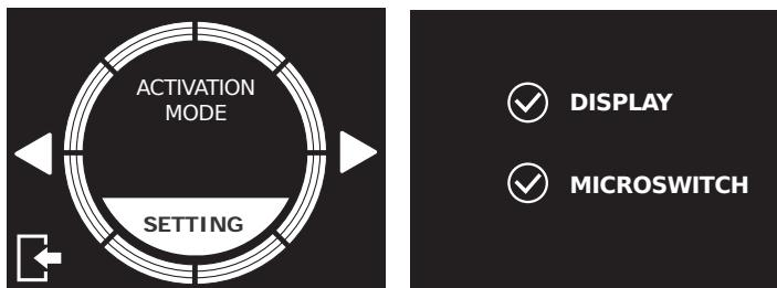
After pressing **SETTING** button, it's possible to choose whether triggering grinding pressing the dose button on the display (**B,L,C,H**) or through the grinding activation button (**6**). It's also possible to select both modes.
